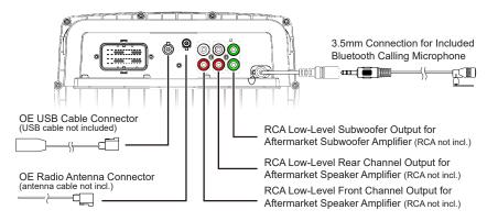
3. Insert and lock the male OEM head unit wire harness connector to the female socket of the included wire harness for HDHU.14. Then, insert and lock the male connector of the HDHU.14 wire harness into the corresponding female socket on the back of HDHU.14.
