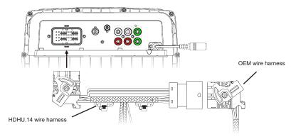
4. If an alternative handlebar integration module other than Scosche is available, skip this step and proceed to step 5. If included, connect the Scosche handlebar integration module to the corresponding 12-pin and 14-pin connectors on the wire harness of HDHU.14.
