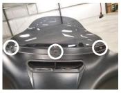
2. Remove four inner fairing bolts using a T27 Torx screw driver. The four inner fairing bolts are located adjacent to each turn indicator mounting bracket and below/adjacent to each speaker. Store these screws in a safe place for re-installation later.
